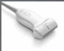
L15-4 ● 15-4 MHz Linear Scan Depth: 6 cm
